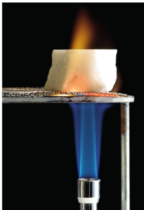
fig A Calcium oxide forms when calcium carbonate (limestone) is heated strongly. If the strong heating is continued, there is no further chemical change, but a very bright glow is seen. This is the origin of 'limelight' – it was formerly used in theatre lighting.
