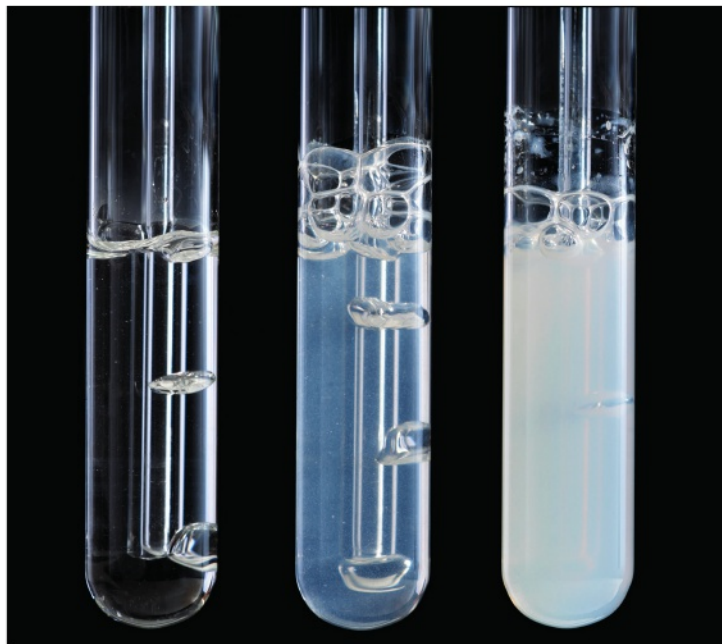
▲ fig A Limewater is a colourless solution. As more carbon dioxide is bubbled through it, the amount of white precipitate increases.
