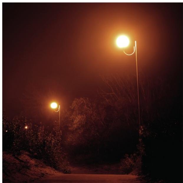
fig C The yellow-orange colour of sodium street lights is the same as the colour of sodium in a flame test.
