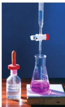
▲ fig C This shows the burette after the titration has been done. Note the white tile and the colour of the phenolphthalein indicator. The pink colour shows that an acid has been neutralised and there is an excess of an alkali.
