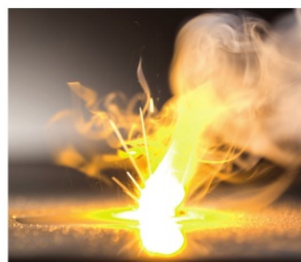
▲ fig B The heat energy from the reaction between these pieces of sodium and water has ignited the hydrogen formed.
