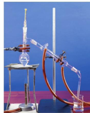
▲ fig B This is just one of the many apparatus set-ups using ground-glass joints.
