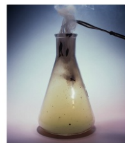
▲ fig B Magnesium burning in chlorine.
