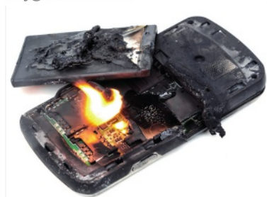
▲ fig A The lithium inside the battery of this mobile phone caught fire.
