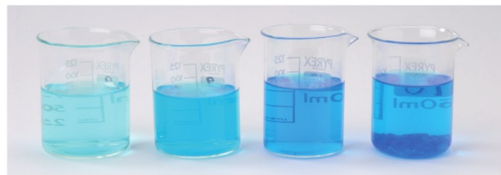
▲ fig A These containers indicate increasing relative solute concentrations by increasing colour intensity. Unfortunately, most solutions we use are not coloured, so we cannot rely on different colour intensities to indicate different concentrations.
