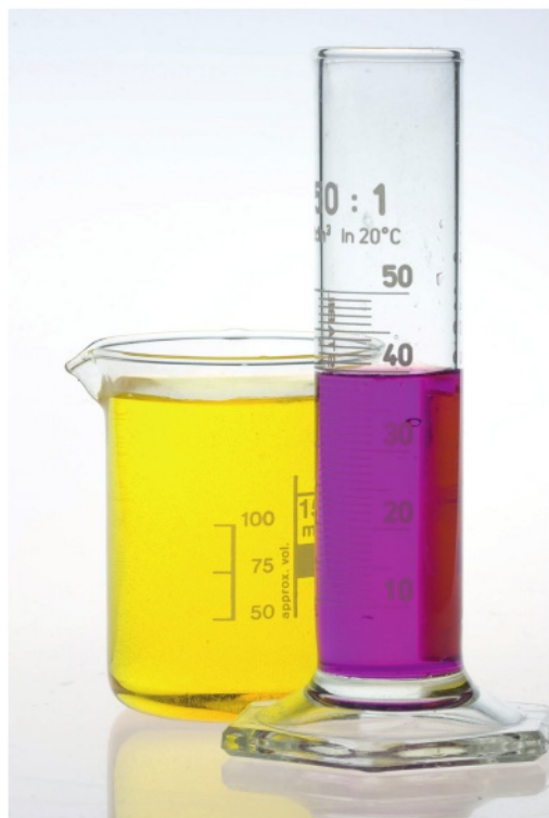
fig B The scale on a beaker is there only as a guide and should not be used to record values to be used in calculations. A measuring cylinder is better for this purpose.
