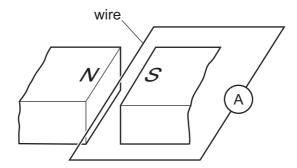
The wire is moved downwards, towards the bottom of the page. A current is induced in the wire.
