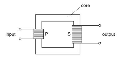
Which equation relates the input and output voltages to the numbers of turns in P and in S?
