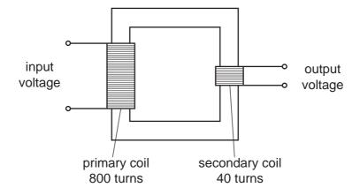
The input voltage is 240 V.
