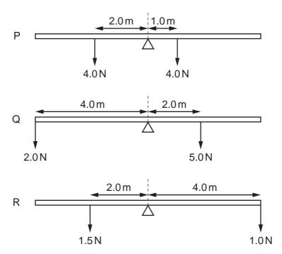
Which beams rotate clockwise?
