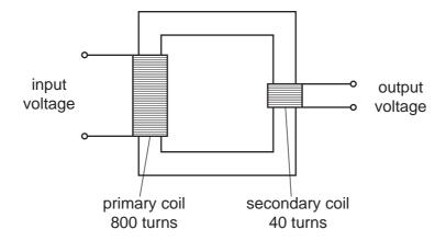
The input voltage is 240 V.
