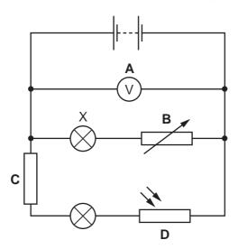
34 In the circuit shown, the current from the battery divides equally between the two lamps. Each ammeter reads 6.0 A.
