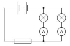
What is a suitable rating for the fuse in this circuit?
