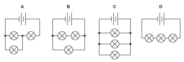
**31** The diagrams show different resistor arrangements.
