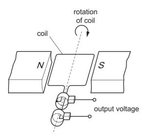
As the coil passes through the position shown, the output voltage is +10 V.
