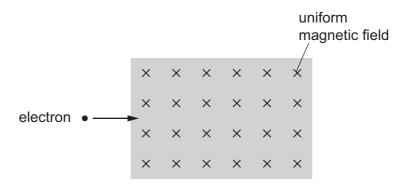
In which direction does a force act on the electron when it enters the magnetic field?
